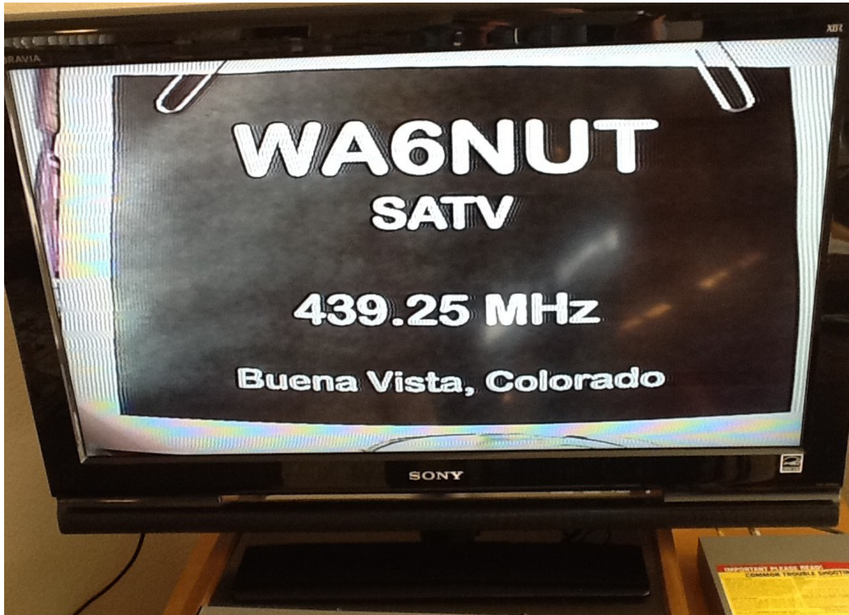
Figure 3: The received ATV image, without the lowpass video filter (it's not SATV) Page 9
